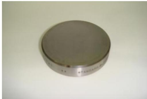
Fig. 1-8 Standardized hardness test block
