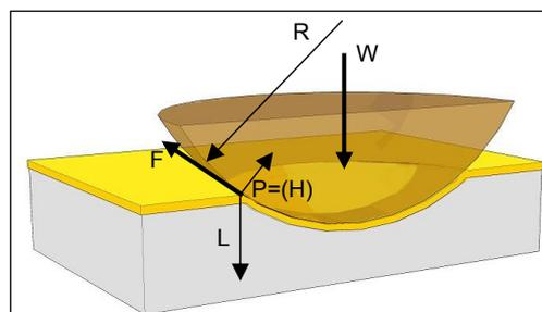
(which affects an interface when the indenter is pressed on the film surface and is used to make scratches) becomes higher than the film adhesion strength, fracturing at the interface occurs.
