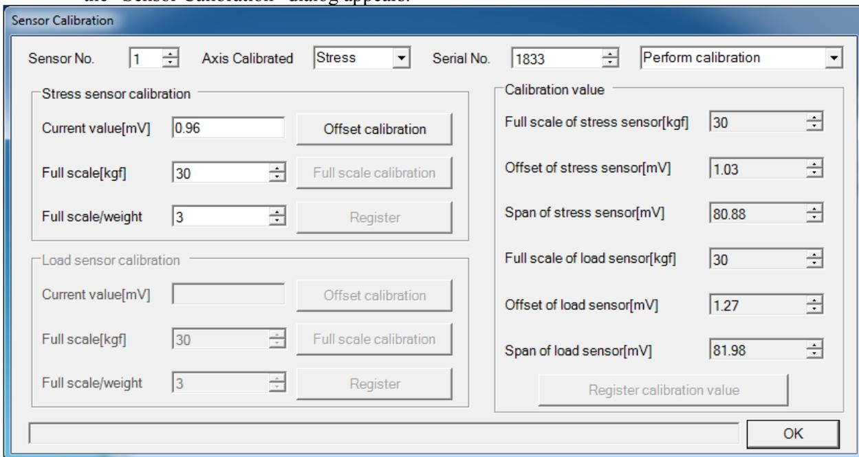
Fig. 11-7 “Sensor calibration” dialog
