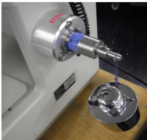
Fig. 11-8 Calibrating the stress axis
