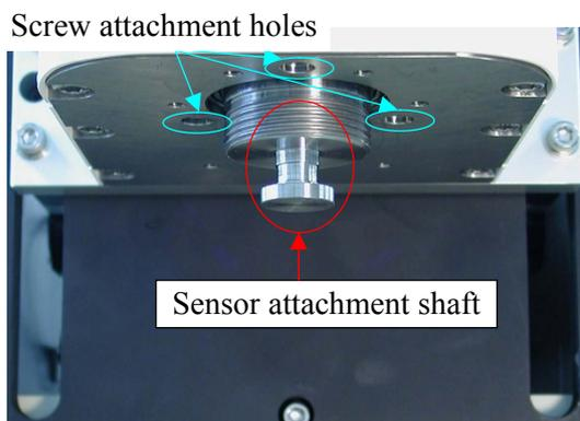
Fig. 5-9 Sensor fixing section
