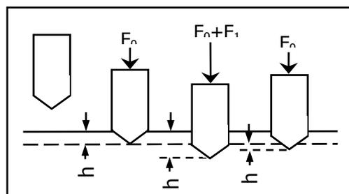
indenter is made of diamond, steel, or cemented carbide balls that have a tip like a cone with an angle of 120 degrees and a radius of 0.2mm. The symbol “HR” is used to express the hardness value and it is standardized in accordance with the type of indenter, initial force, and test force. An initial test force of 29.42N (3Kgf) is applied to measure the Rockwell superficial hardness of a material.
