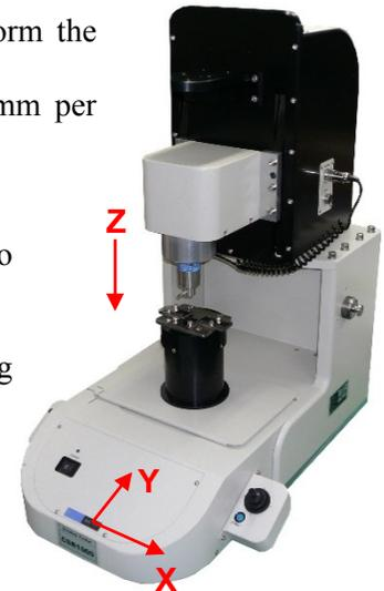
Fig. 7-5 X-, Y-, and Z-axis directions
