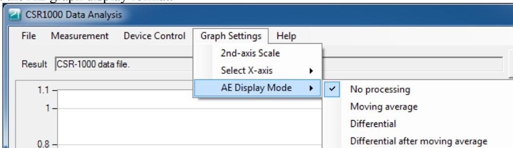
Fig. 8-24 Selecting the “Display AE data” submenu
