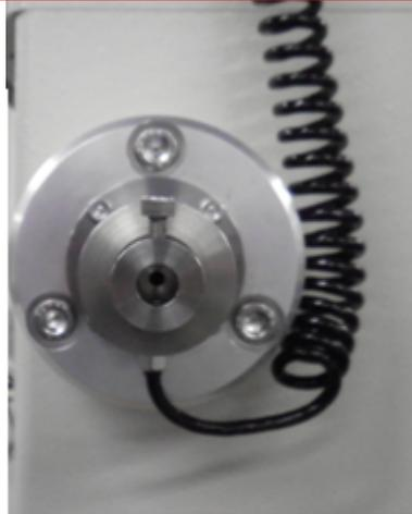
Fig. 11-5 Attaching the sensor
