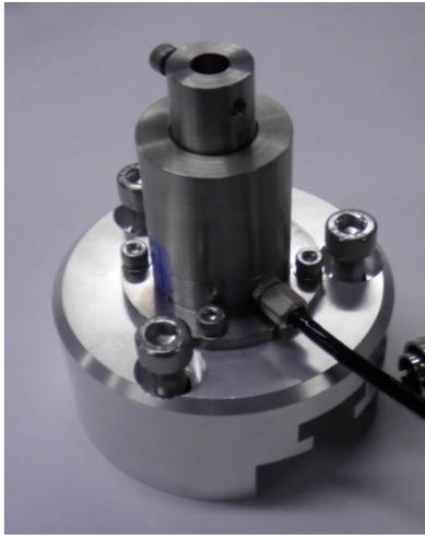
Fig. 11-2 Sensor (attached with high-load block)
