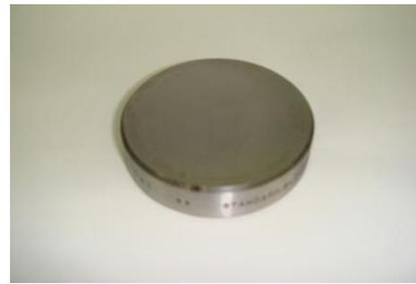
Fig. 9-2 Standardized hardness test block
