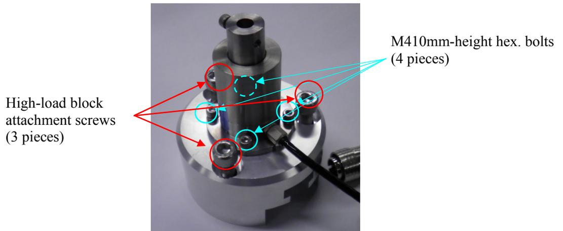
Fig. 5-8 Attaching the sensor to the block
