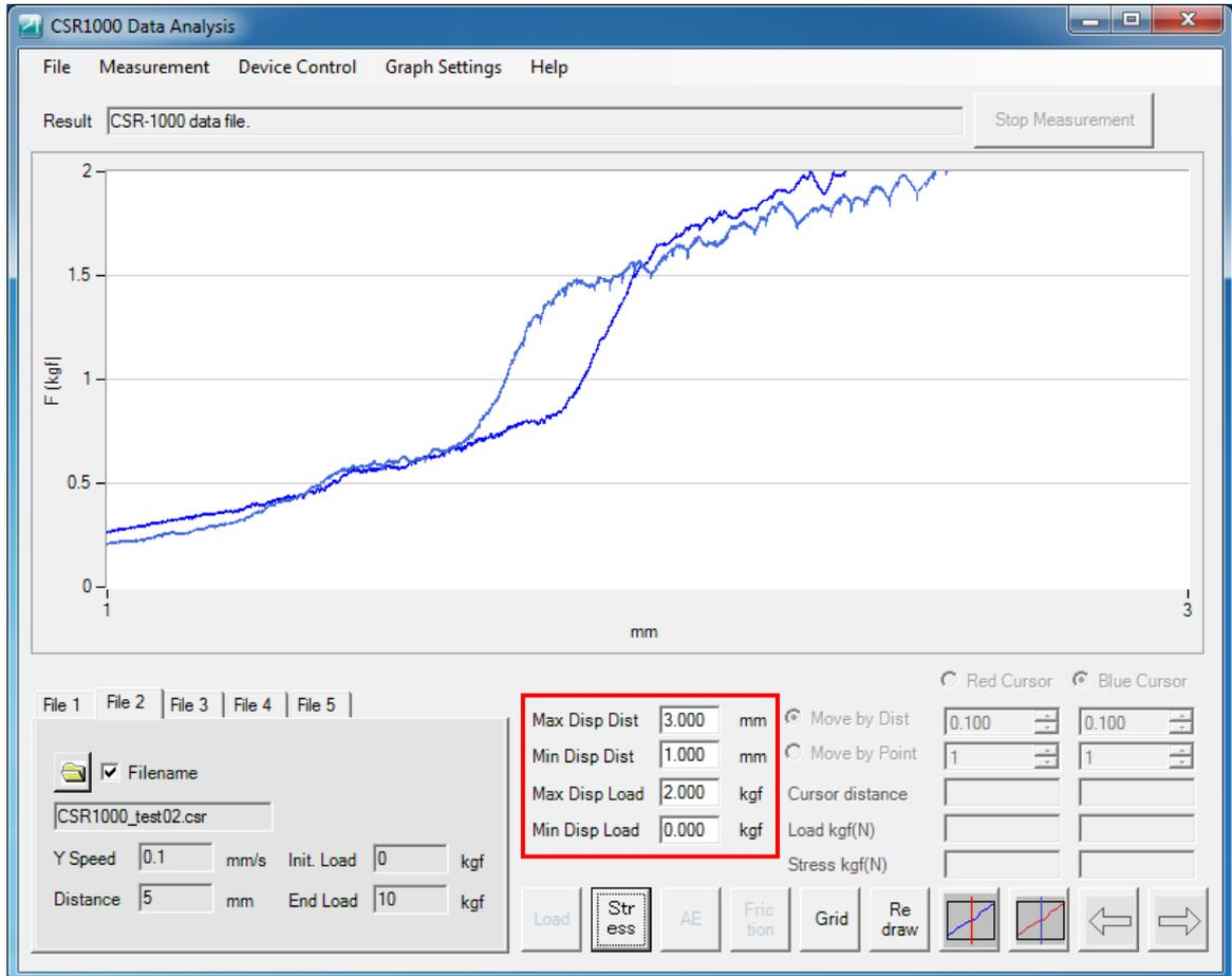
Fig. 8-10 Example of enlarged display by specifying both distance and load values
