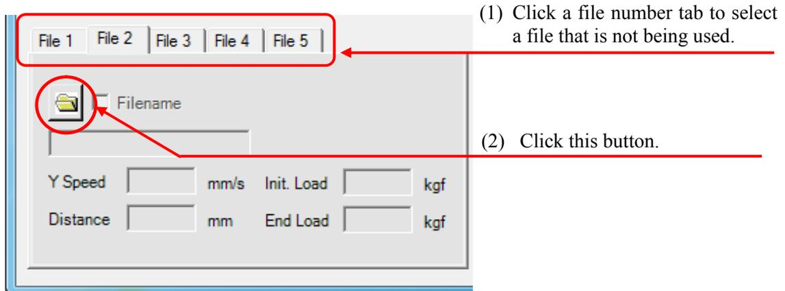
Fig. 8-8 Selecting a file for overlaying data
