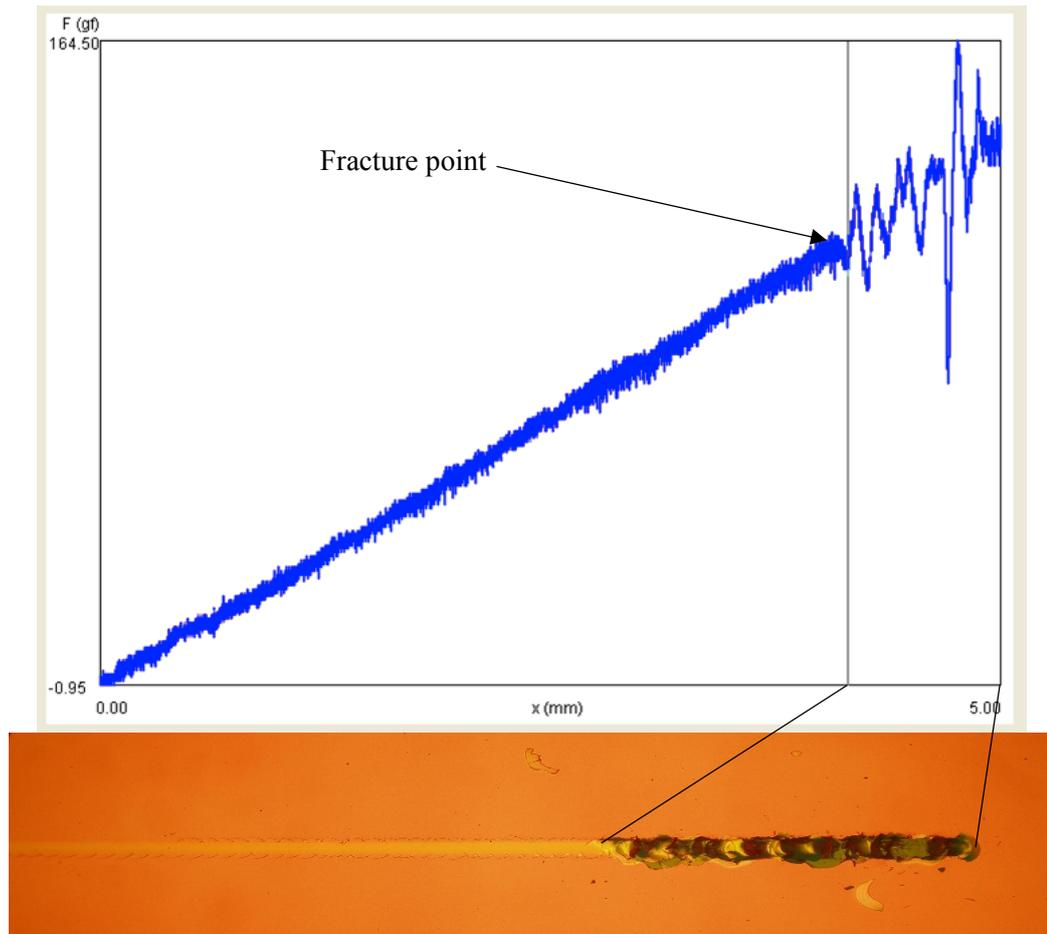
Fig. 3-3 Comparison between measured data graph and optical thin-film fracture surface observation photo through a metallurgical microscope
