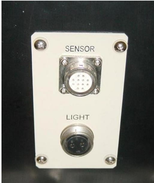
Fig. 5-11 SENSOR connector
