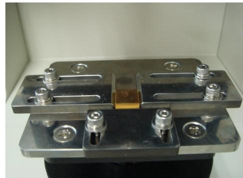
Fig. 5-17 Fixing a sample on the stage
