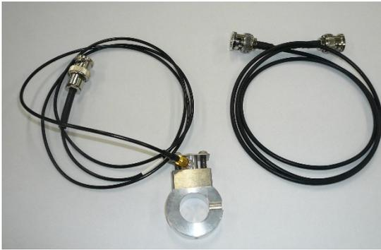
Fig. 1-5 AE sensor and BNC cable
