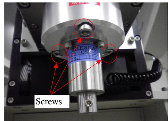
Fig. 5-10 Attaching the sensor
