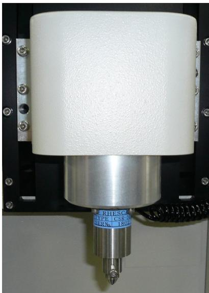
The sensor is attached to the head part in the upper front side of the main unit (see Fig. 2-1-(3)). The diamond chip is attached to the sensor. To attach and detach the sensor, see “5-4 ”.
