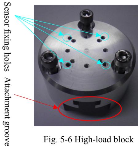
Fig. 5-6 High-load block
