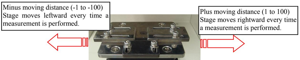
Fig. 7-6 Moving direction of stage for repeat measurements
