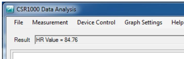
Fig. 9-5 Hardness measurement result
