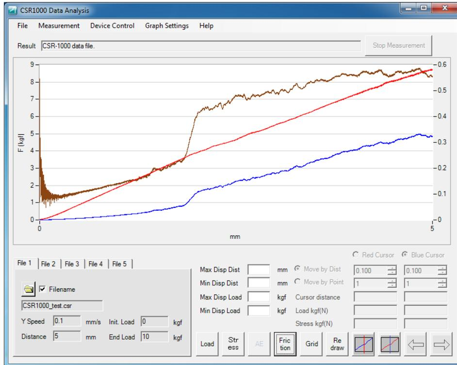
Fig. 8-7 Example of graph display with friction coefficient data
