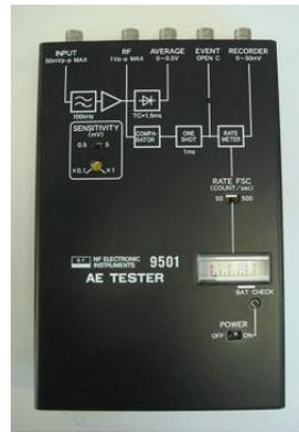
Fig. 1-6 AE sensor amplifier
