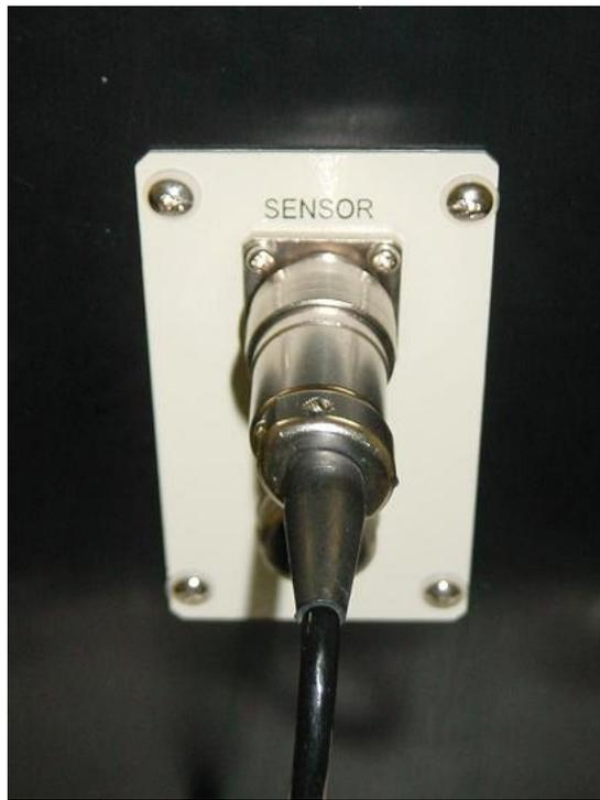
Fig. 5-12 After connecting the cable to the SENSOR connector
