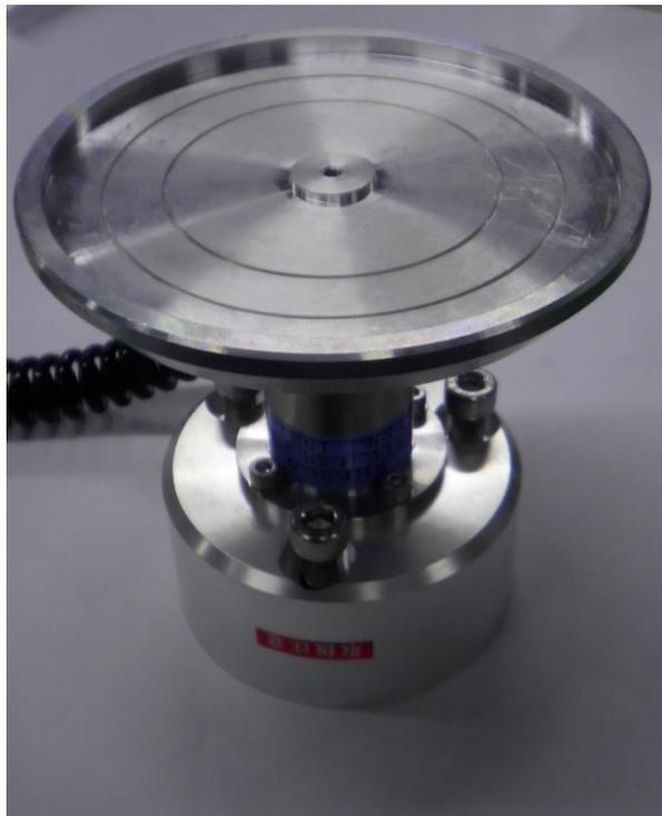
Fig. 11-10 Sensor and calibration flange
