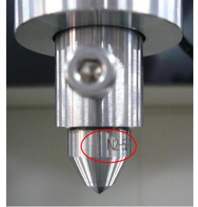
Fig. 5-15 Sensor attached with chip
