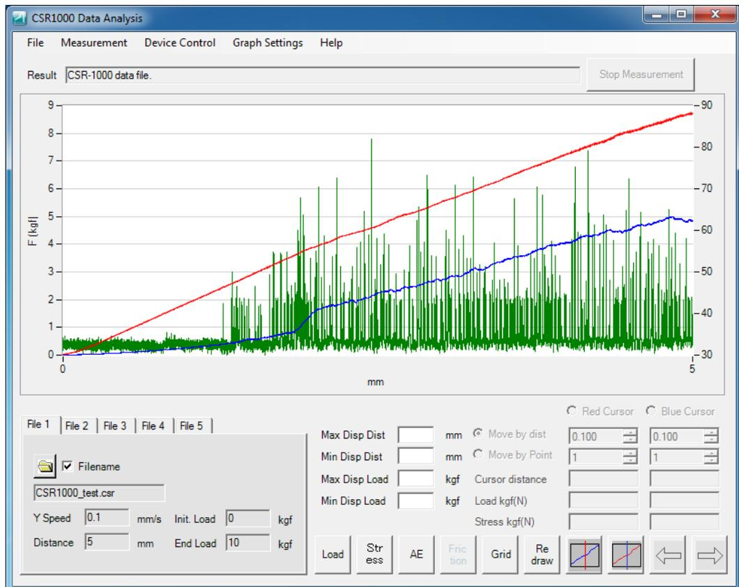
Fig. 8-26 Example of graph when “Moving average” is selected
