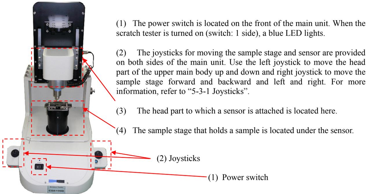
Fig. 2-1 Front view of main unit
