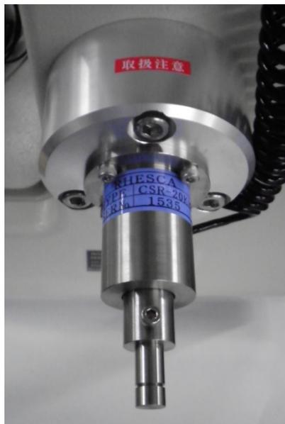
Fig. 11-6 Sensor attached with Y-axis calibration jig
