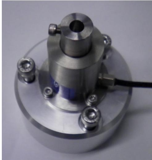
Fig. 11-9 Sensor (high-load block)
