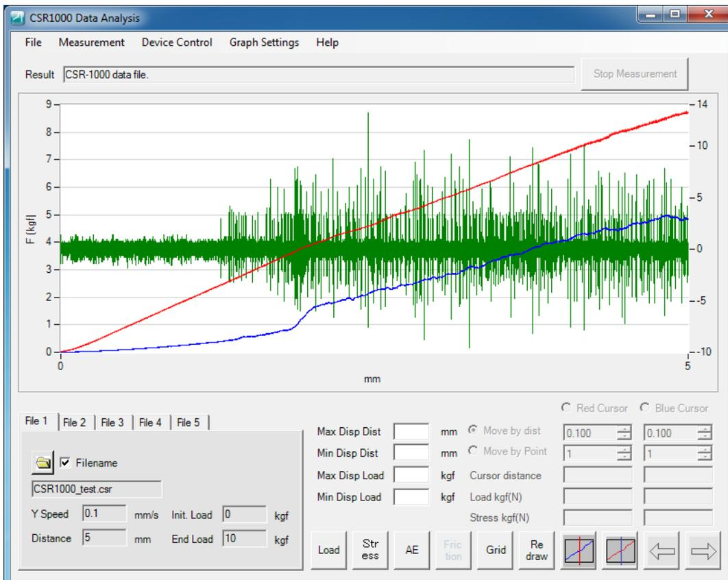
Fig. 8-28 Example of graph when “Differential after moving average” is selected
